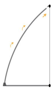
**4.** Flex the rod made up of three tubes until it is inserted into the connection detail attached to the upper profile.
