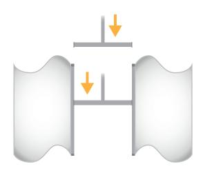
**1.** Open the two aluminum snap profiles, insert the print and then close the profiles again
