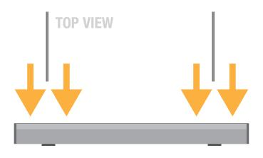
4. Insert the composite rods in the pedestal's holes. WARNING - make sure that the rods are perpendicular to the ground
