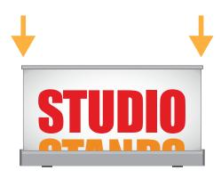
**3.** Remove the locking key of the print winding mechanism then rewind the graphic inside the structure.
