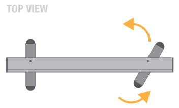
**3.** Rotate the feet, attached to the lower part of the frame, in a perpendicular position compared to the structure.
