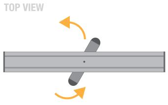
**3.** Rotate the foot, attached to the lower part of the frame, in a perpendicular position compared to the structure.
