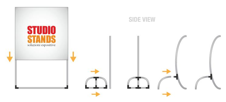
**2.** Apply the print by inserting the structure into the slot, tension and secure with the existing Velcro.
