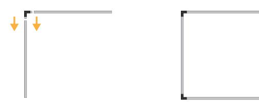
1. Compose the structure by simply joining together tubulars and fittings according to the chosen configuration.
