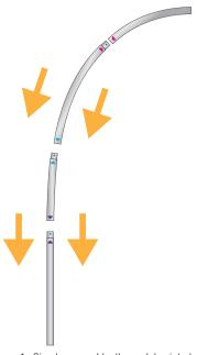
1. Simply assemble the rod by interlocking, following the numbering of the stickers on the tubulars  $\,$
