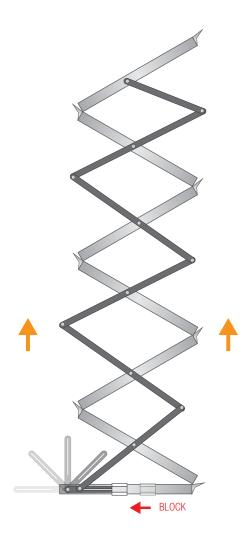
**2.** Extend the structure vertically; lock in position by acting on the sliding block on the side of the pedestal
