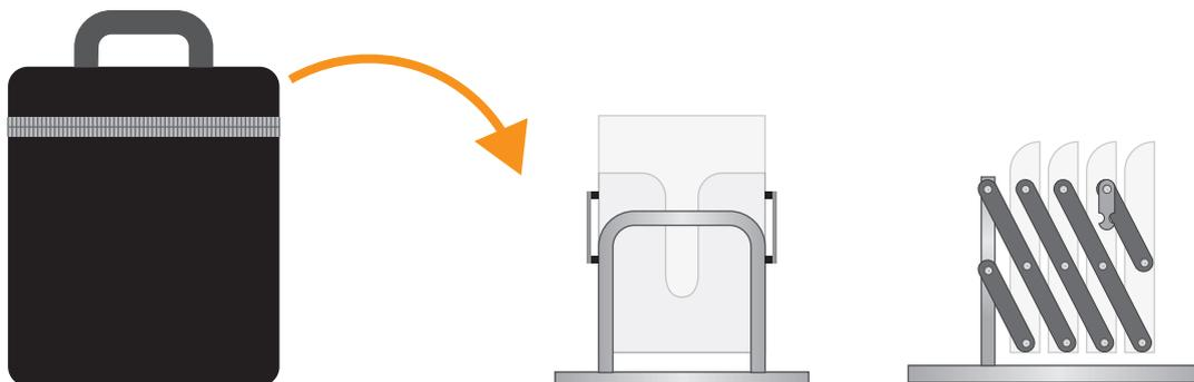
1. Remove the display from the transport case
