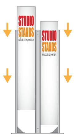
**4.** Insert the printed panels into the appropriate shaping of the shoulders by simply sliding them.
