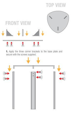
$\pmb{3}.$  Apply the bracket to the upper end of the shoulders and secure with the screws supplied.
