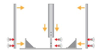
**2.** Apply the shoulders to the corner brackets and secure with the screws supplied.
