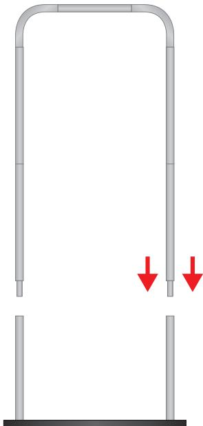
3. Join the interlocking parts together
