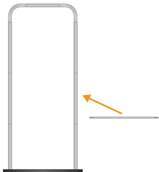
4. Screw the intermediate crosspiece to ensure greater consistency to the structure
