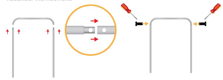
1. Join the curved rod with the 2 vertical rods and secure with the screws supplied
