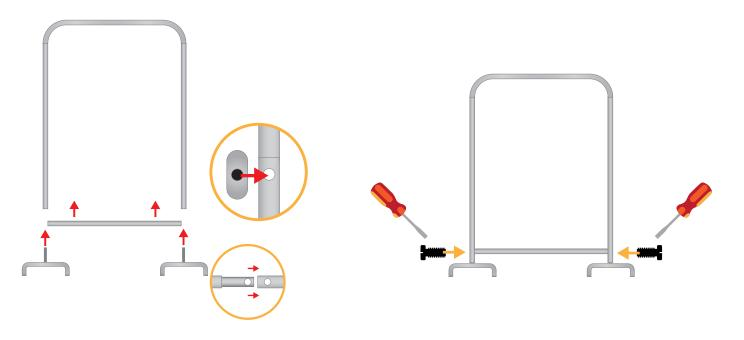
2. Insert the pin of the feet into the vertical rods, position the horizontal rod and secure with the screws supplied
