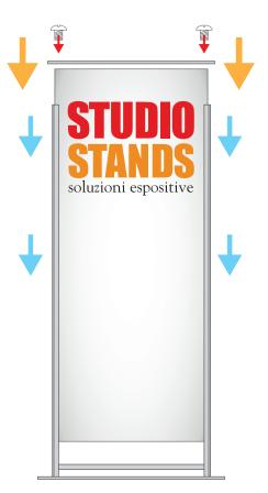
${\bf 4.}$  Insert the printed panels into the appropriate shaping of the shoulders by simply sliding them.
