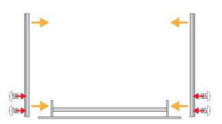
**1.** Apply the shoulders to the corner brackets and secure with the screws supplied.
