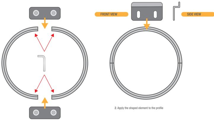
1. Insert the fittings into the appropriate shapes to join the parts together and lock in position with an Allen  $\ensuremath{\mathsf{key}}$
