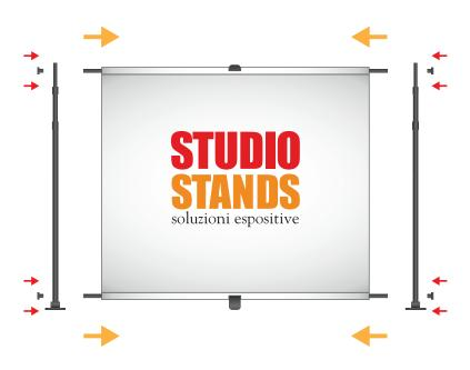
**10.** Apply the print to the floor lamps using the butterfly screws (long) supplied
