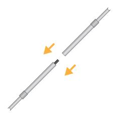
2. Compose the horizontal rods by joining together the telescopic rods shaped at the top (adjust the length by acting on the knurled parts)
