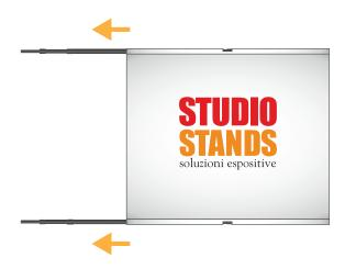
**8.** Assemble the horizontal telescopic rods and insert them into the slots of the press.
