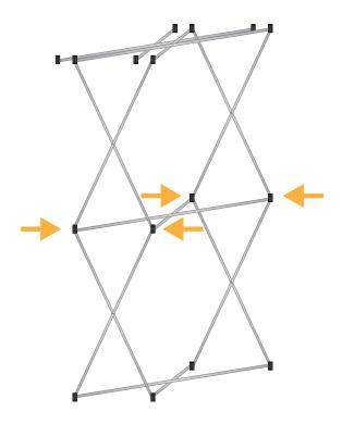
2. Fully extend the structure by pushing the vertical elements towards each other.
