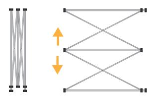
1. Keep the structure in a vertical position and open like an umbrella.
