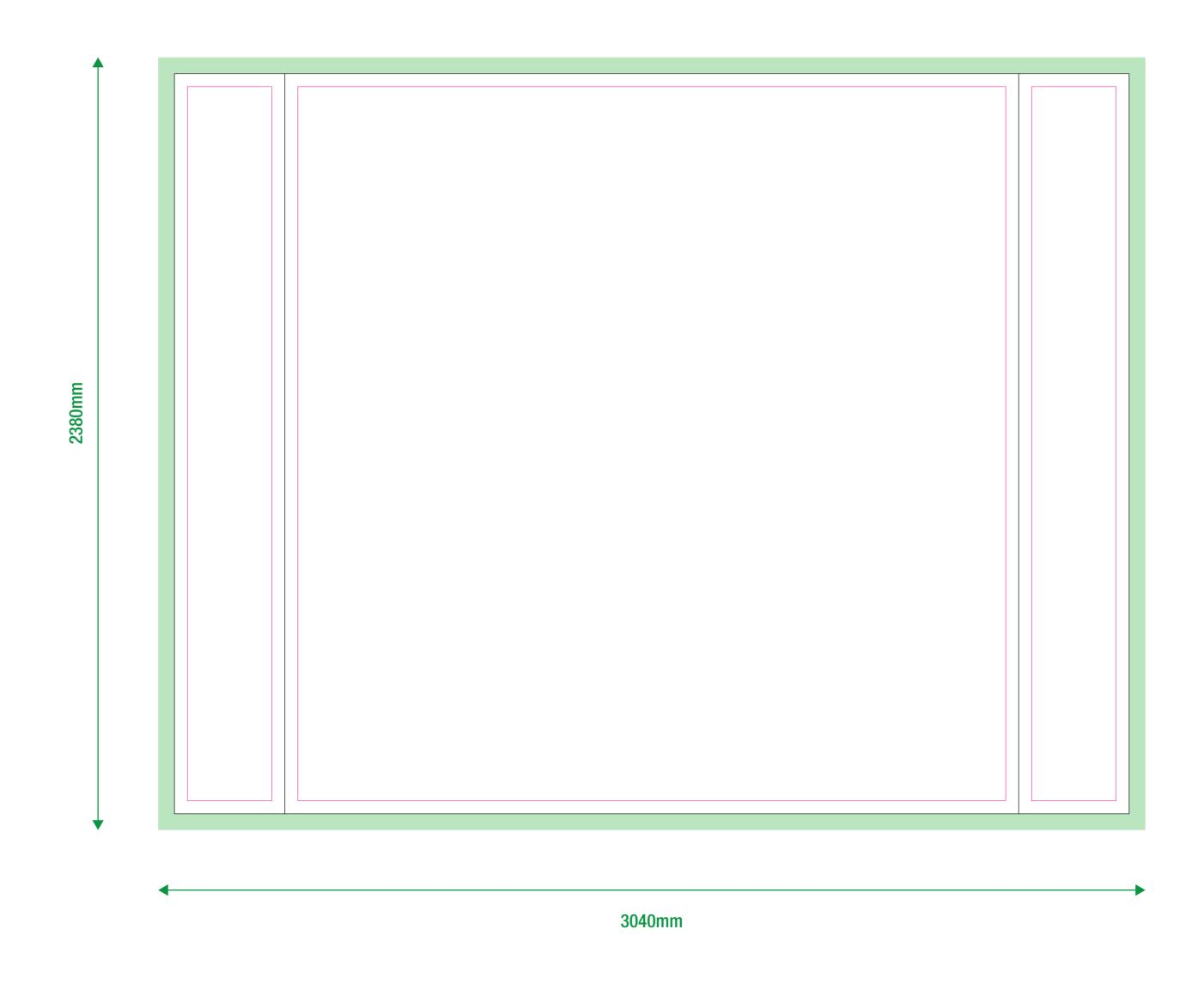
Velcro profiles to be applied to the back of the print thickness approx. 4cm
