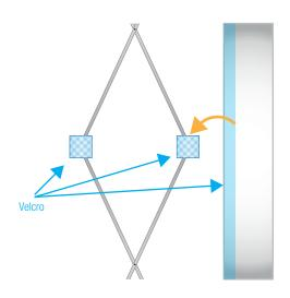
**4.** Fix the graphics laterally by acting on the Velcro present on the joints on the sides of the structure.
