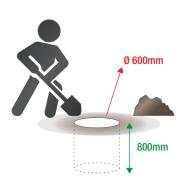
1. Dig a 600mm diameter hole with a depth of 800mm
