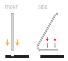
**1.** Insert the support rod into the shape of the pedestal and secure with the screws supplied
