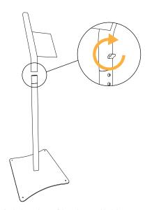
**4.** Apply the end part of the column and lock in position by acting on the butterfly screw
