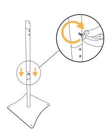
**3.** Insert the central segment and lock in position by acting on the throttle screw to lock in position
