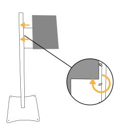
${\bf 5.}$  Insert the panel and lock using the screws
