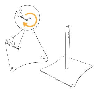
2. Insert the screws, apply the first column segment and use the Allen key on the screws to lock in place
