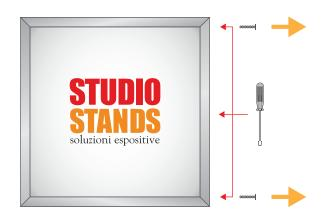
**1.** Remove the screws on two sides of the box (the sides must be contiguous)
