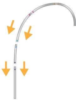
1. Simply assemble the rod by interlocking, following the numbering of the stickers on the tubulars ATTENTION - the number of tubulars varies depending on the format chosen
