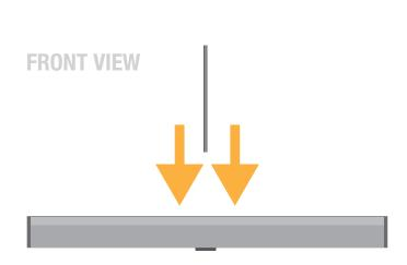
4. Insert the composite rod into the hole in the structure. ATTENTION - make sure the rod is perpendicular to the ground
