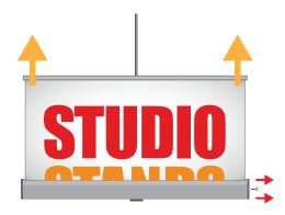
**5.** Remove the locking key of the print winding mechanism and then remove the graphic from the structure by simply pulling. Fix the rod to the upper profile.
