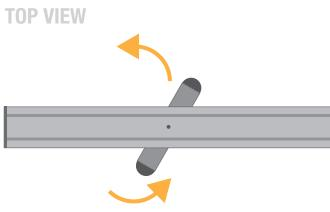
**3.** Rotate the foot at the bottom of the display stand to a perpendicular position with respect to the structure.
