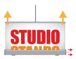
**5.** Remove the locking key of the print winding mechanism and then remove the graphic from the structure by simply pulling. Fix the rod to the upper profile.
