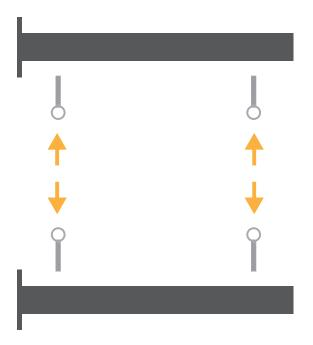
**1.** After fixing the black tubes to the wall, apply the four eyelet screws in the appropriate holes.
