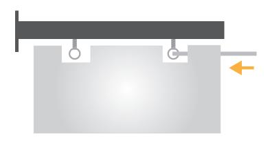
**2.** Insert the metal rod into the upper slot of the print and into the screw eyelets.
