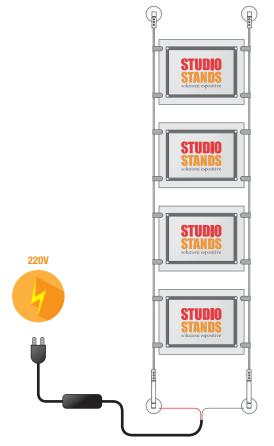
**10.** To turn on the LED panels, simply connect the power supply to a normal 220V socket.
