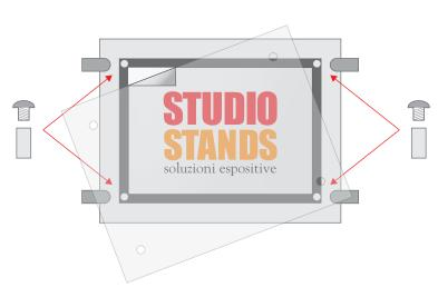
**9.** To position the prints, remove the spacers on the back of the display, remove the protective panel, position the print and reapply the spacers
