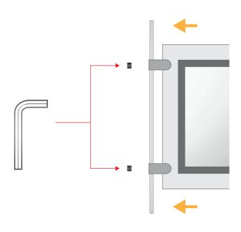
**7.** Position the communication holders at the desired height by inserting the cables into the perimeter attachments of the display, then secure by repositioning the pegs removed previously.
