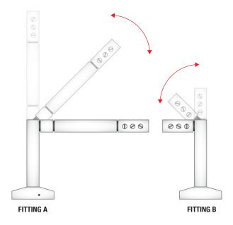
**1.** Drill the wall/ceiling/floor according to the chosen configuration; apply the articulated supports using screws and plugs, positioning them at the necessary distance imposed by the dimensions of the communication holders.
