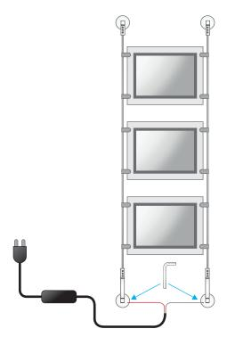
8. Insert the power cables into the appropriate holes and lock them by acting with the Allen key on the bolt present
