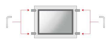
**6.** Using an Allen key, remove the small screws present in the perimeter attachments of the backlit communication holders.
