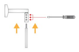
**3.** Insert the "stripped" cable into the hole in fitting B and secure by acting on the screws present **- Attention -** Tighten well to prevent it from coming off with the weight of the backlit communication holders.
