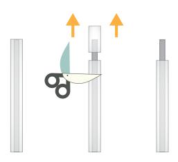
2. Using scissors/nippers, remove the end part of the rubber protection of the steel cable
