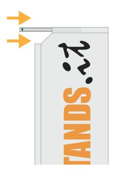
**1.** Insert the horizontal rod into the slot of the print.
