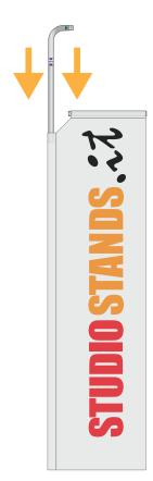
${\bf 3.}$  Insert the vertical rod into the slot of the press and join the fitting with the horizontal rod inserted previously
