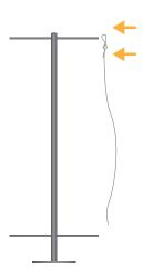
**3.** Apply the steel cables with the loop already prepared to the upper crossbar
