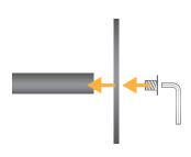
**1.** Join the circular base to the vertical pole, fixing the parts with the screw and Allen key supplied.
