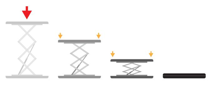
2. Apply pressure on the support surface until the DESK QUICK starts to close.
