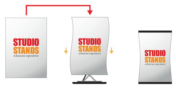
3. Insert the fabric print into a "bag" and insert the silicone profiles present in the appropriate slots. NOTE: DESK QUICK can be opened and stored with the print pre-installed.
