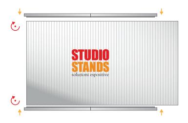
${\bf 2.}$  Wrap the printed profile so that the Velcro bands coincide, then apply the top in the same way
