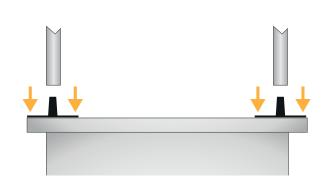
4. Insert the tubes into the previously applied couplings
