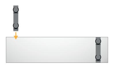
**2.** Apply the attachments for the tubes to the back of the Crowner with double-sided tape and the self-tapping screws supplied.
