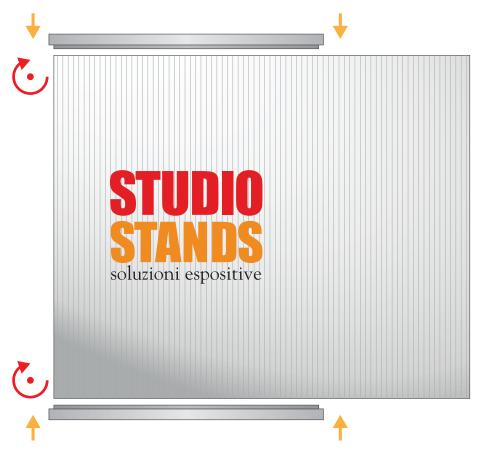
${\bf 1.} \ {\bf Wrap \ the \ printed \ panel \ making \ the \ Velcro \ profiles \ of \ the \ top \ and \ base \ coincide \ with \ those \ applied \ on \ the \ back \ of \ the \ graphics.}$
