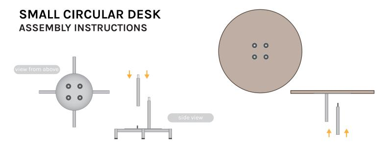
1. Apply the aluminum tubes to the base following the order of the numbered stickers
