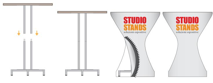
3. Join the support surface to the base
