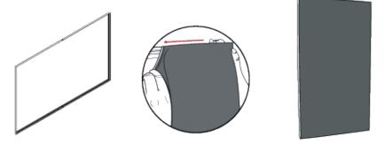
**6.** Apply the print with silicone profile to the structure
