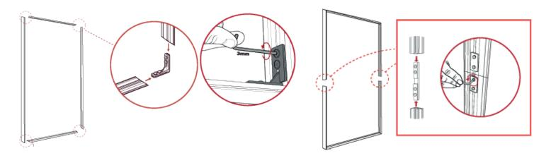
1. Join the profiles together with the appropriate fittings and lock with an Allen key
