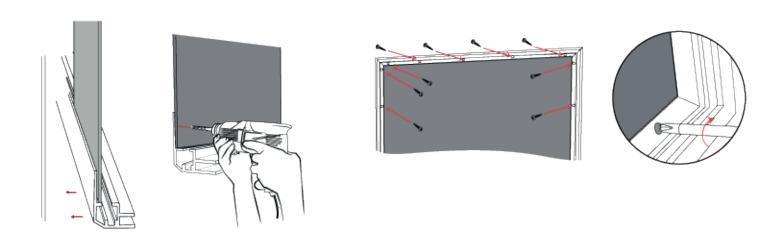
2. Position the panel (composite aluminum recommended material - the panel must be 25mm smaller than the frame) then secure to the wall using the self-tapping screws position in correspondence with the appropriate holes on the profiles
