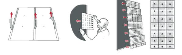
3. Apply the LED backlight modules to the panel using the double-sided tape on the back of the modules
