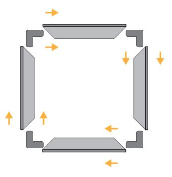
1. Insert the interlocking fittings into the components to form the frame
