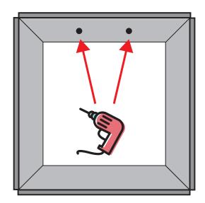
$\boldsymbol{3.}$  Using a drill, make holes in the structure for wall mounting.
