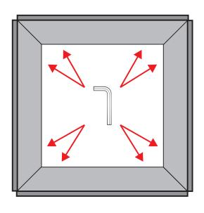
2. Use an Allen key to tighten the nuts on the fittings
