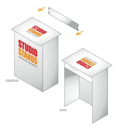
2. Position the support panel in the rear part, joining the two side rails
