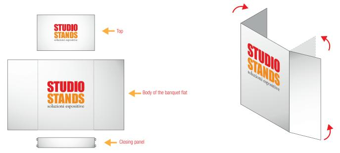
1. Arrange the die-cut panel in a "U" shape
