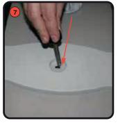
Secure the base covers with the 4 base screws removed previously.
