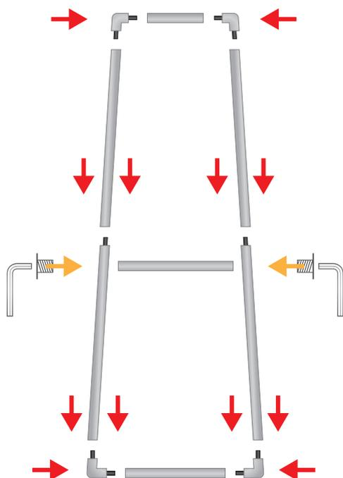
1. Compose the two semi-arches of the structure by joining the aluminum tubes together following the numbering of the stickers present
