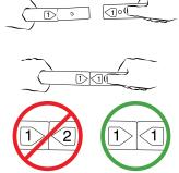
join the components together by associating the numbers together to compose the structure
