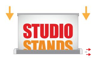
**3.** Remove the locking key of the print winding mechanism then rewind the graphic inside the structure.
