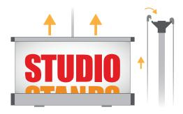
**9.** Extract the print from the structure until applying the shaped profile to the rod (repeat the operation for double-sided setups).
