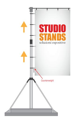
7. Connect the composite rings on the telescopic rod to the eyelets of the press and gradually extend the central pole. (a counterweight is supplied to be applied to the last ring at the base of the print to ensure better visibility)
