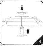
4. Assemble the upper connection-unit, unfolded-base and section(as step-3) together
