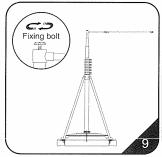
9.Connect the horizontal-pole and vertical-pole 10.Every hook with the banner should be with the upper-screw.
