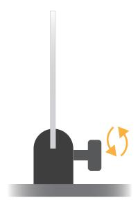
**4.** Place the screws into the base and panel, screw them until they are completely fixed.
