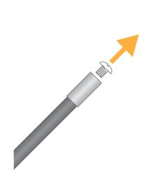
**2.** Remove the screw at the bottom of the telescopic pole.
