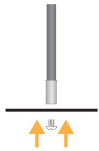
**3.** Insert the screw into the hole in the metal stand and attach the rod to the base.
