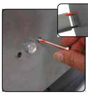
**3.** insert screws to holes on base and then fasten them to bottom of shaft.
