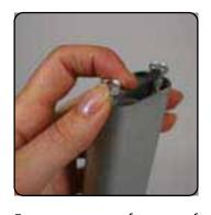
**5.** unscrew screws from top of shaft
